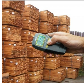
Measuring Moisture Content in Wood
