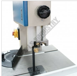
Height Adjustment handle for Top Blade Guide
