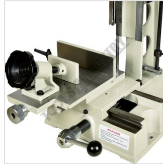
Dovetail Slideways on Work Table
