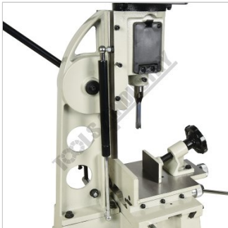
Gas Strut to Counterbalance Head Weight
