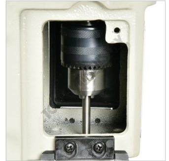
Drill Chuck Access
