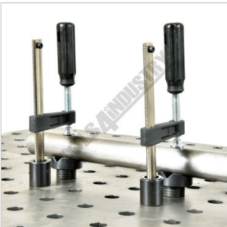
Clamps Shown Clamping Round Tube
