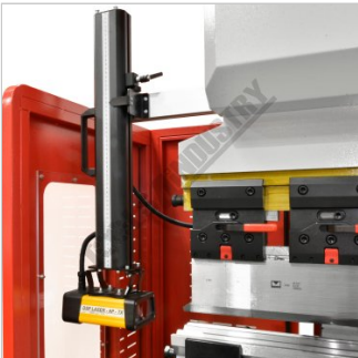
Laser Guarding System with Alignment Guide
