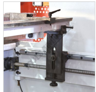
Linear Guideway Ballscrew Backgauge
