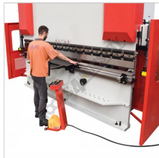
Laser Guarding system In Use
