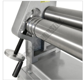
Rear Roll Height Adjustment And Roll Grooves
