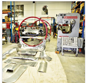
All Car Parts Made on Power Hammer
