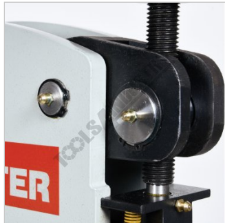
Head Pivot Points with Grease Nipples
