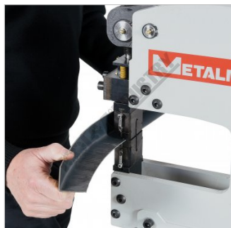
Shrinking Dies In Action 2mm Mild Steel
