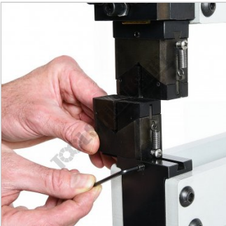
Dovetail Dies For Quick Self Aligning
