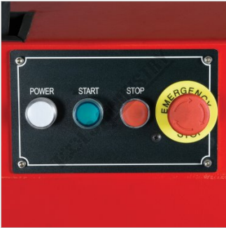
Power Control Panel
