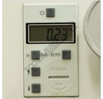
Digital Readout for Quill Depth
