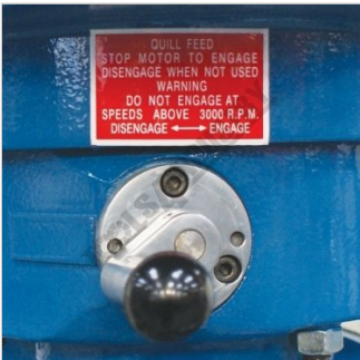
Feed Engage Disengage Drive
