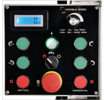
Control Panel With Digital Speed Readout
