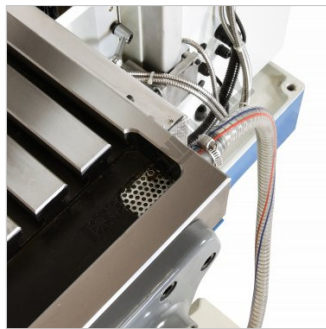
Work Table Coolant Return
