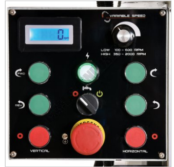
Control Panel With Digital Speed Readout
