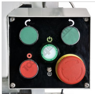
Horizontal Spindle Control Panel
