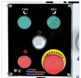
Forward Reverse ON OFF and Emergency Switches
