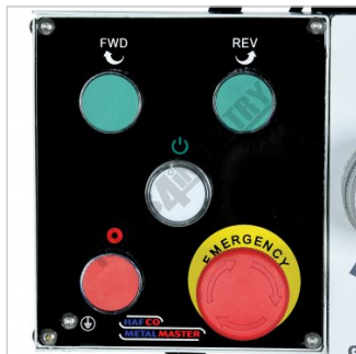
Forward Reverse ON OFF- Emergency Switches
