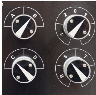
Gearbox Feed Controls
