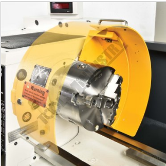
Chuck Guard with Safety Micro Switch
