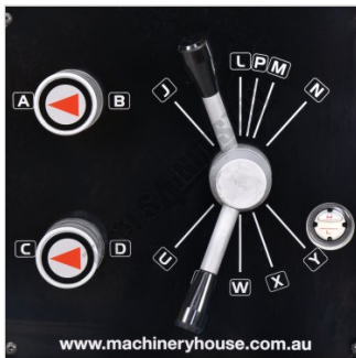
Feeds and Threads Gearbox Levers
