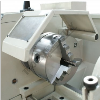
Chuck Guard With Safety Micro Switch
