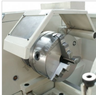
Chuck Guard With Safety Micro Switch
