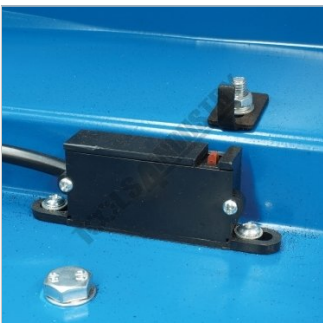
Safety Micro Switch on Pulley Guard
