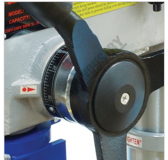
Drilling Depth Stop Setting With Scale
