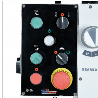
Control Panel with Tapping Function
