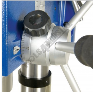
Drilling Depth Stop Setting With Scale
