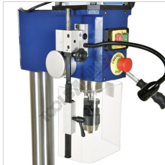
Drill Chuck Safety Guard with Micro Switch
