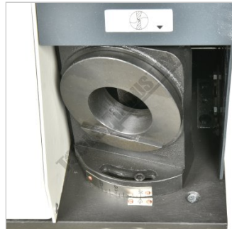
Drill Angle Setting at 90 Degrees
