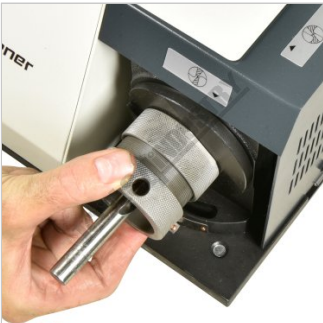
Sharpening Drill Bit Station 1
