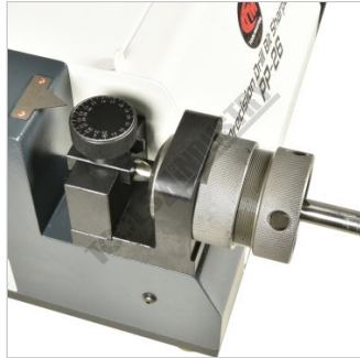
Drill Setting Gauge Shown with 13mm Drill
