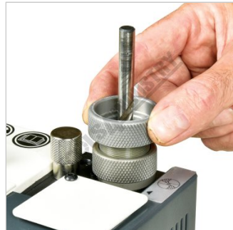
Grinding Split Point Station
