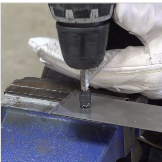
Push Down Ready For Drilling
