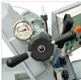
Blade Tension System With Gauge
