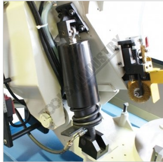
Hydraulic Feed Ram with Spring Dampener
