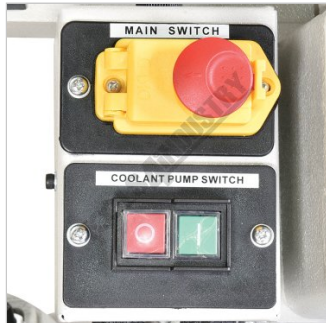
Main Switch and Coolant Pump Switch
